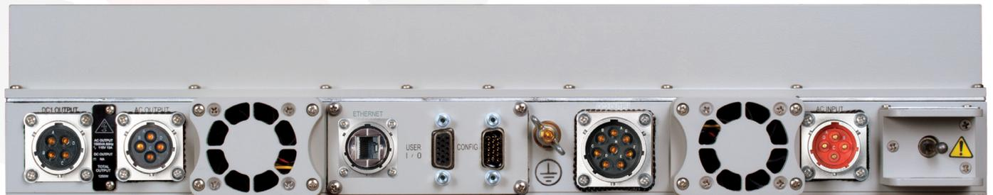
DC1 Output Option    AC Output    Exhaust Fan    Ethernet Port Option    User I/O    CONFIG Port    Ground Stud (1/4-20)    DC2 Output Option    Exhaust Fan    AC Input    AC Circuit Breaker
