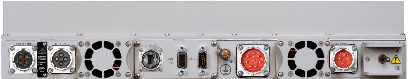
DC1 Output Option    AC Output    Exhaust Fan    Ethernet Port Option    User I/O    CONFIG Port    Ground Stud (1/4-20)    DC Input Option    Exhaust Fan    AC Input    AC Circuit Breaker
