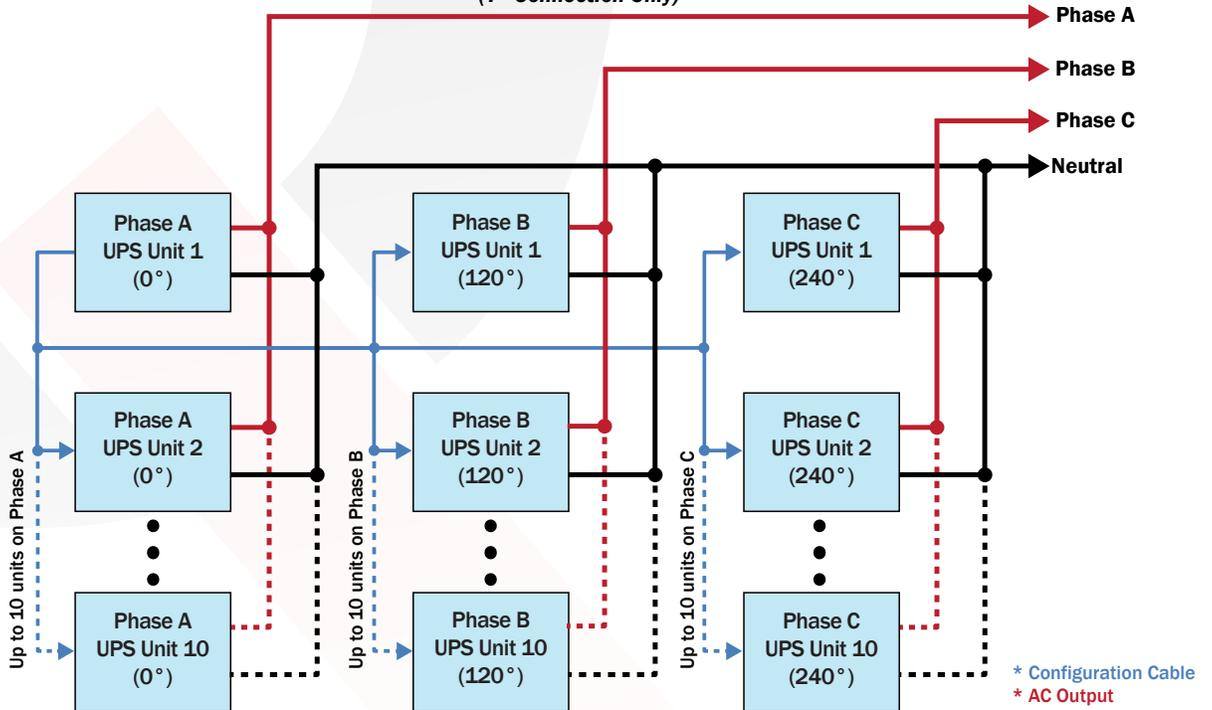
\* Contact factory for system specific configuration cables.
