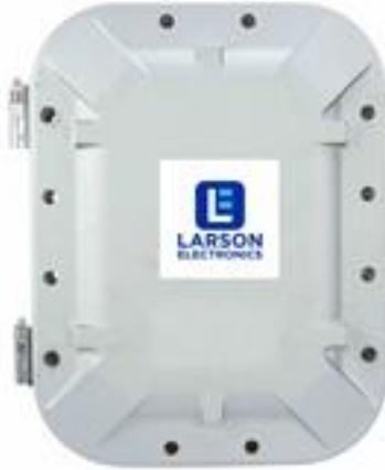
The Larson Electronics EPPB-TWI-MOD7 Explosion Proof Power Distribution Box is designed for safe disconnection of power in combustible work sites. Equipped with a 3-pole disconnect/isolator switch, the unit is rated 400V AC three phase 50 Hz (40 amps max). The IP66-rated enclosure is constructed of copper-free aluminum with stainless steel hardware (SS 304/316).
