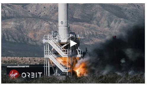
a custom layered wrap that was able to protect the steel structure from the 5 minute exposure to temperatures nearing 6,000 degrees and 70,000 foot pounds of thrust. Sun Fire Defense was able to protect these costly structures from incredibly high heat and thrust exposure and allowed the rocket launch structures to be reused over and over without damage.
