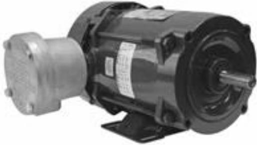
The Larson Electronics EXP-MTR-1P-230-1.5HP-1.8K-56H Explosion Proof Motor is recommended for use in Class I, Divisions 1 & 2 Groups C, D and Class II, Divisions 1 & 2 Groups E, F, G rated work sites. The 1.5 HP unit is compatible with 230V AC single phase 60 Hz and offers 7.8 FLA. This Class F insulation rated explosion proof motor features a NEMA 56H motor frame and can be installed with industrial systems via an integrated mounting foot.
