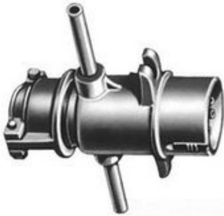
The EPP-200A-3W4P-DW from Larson Electronics is an Explosion Proof Interlock Receptacle that is rated for Class I Divisions 1 & 2 Groups C & D, Class II Divisions 1 & 2 Groups F & G and Class III hazardous areas. This explosion proof cord cap has a voltage rating of 600V AC and 250V DC as well as having a current of 200 amperes. The EPP-200A-3W4P-DW is a 3-Wire, 4-Pole receptacle and can be used in damp, wet and corrosive areas both indoors and outdoors.
