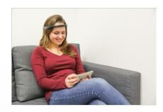
Focus FAMILY is a wearable device that can monitor, visualize and analyze brainwaves. It draws inspiration and techniques from neurofeedback training algorithms. This method improves an individual's everyday focus level by training specific brainwave frequencies.
