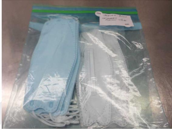
Test Substances Received: Treated – Blue Mask (Left), Control – White Mask (Right)
