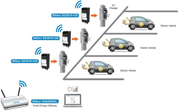
The Billion ZigBee SG3010-iCB can be installed in the EV charger and transfer data to the ZigBee smart energy gateway in order to manage the electrical consumption of EVs.
