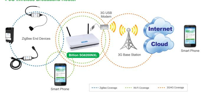
The Billion SG6200NXL functions as a 3G wireless broadband router as well. Users can connect to Internet services by plugging a 3G modem into this router without the need for access to a fixed-line network.
