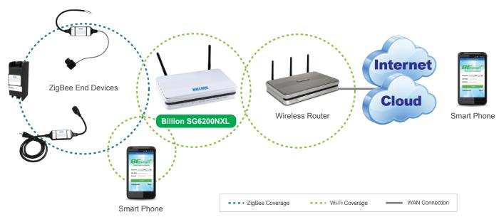
The Billion SG6200NXL can function as a wireless AP and wireless client at the same time, enabling data collection from any ZigBee end devices via a ZigBee wireless network for energy management. It can also serve as a wireless bridge to further connect with an existing wireless gateway.
