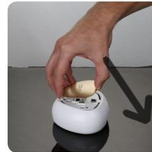
Place the new colored plate on the top of the Covr Point, aligning the guide pins on the plate with the holes in the Covr Point
