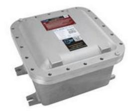
The EPL-AEB-12.12.8-10X1WE from Larson Electronics is an Explosion Proof Enclosure that provides operators with a Class I and II, Divisions 1 and 2 cast aluminum enclosure designed to hold electrical equipment up to 12" by 12" by 8" in size. Equipped with ten, 1" NPT hubs, this explosion proof enclosure is ideal for indoor or outdoor applications where flammable vapors, gases, or dusts exist or stand the potential to exist.
