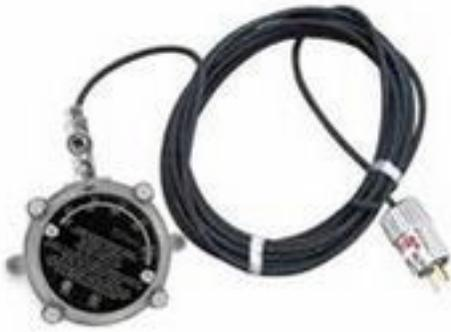
The Larson Electronics EXP-TSTAT-120.240-86F-6C-EPP explosion proof thermostat is designed for temperature control in industrial facilities where flammable gases, vapors or dust are or may be present. This device is adjustable using a set point knob system, which is powered by an SPDT snap action switch. Equipped with a 6-foot 16/3 SOOW cord and an explosion proof cord cap, the unit features a temperature limit range of -49°F to 176°F (-45°C to 80°C) and is rated at 120/240V AC (maximum).
