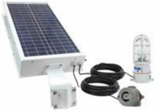
**The Larson Electronics AVL-NVG-SOL-L810-LED-V1-30C Solar LED Strobe Light is an FAA AC 150/5345-43 Compliant unit with applications in aviation and harsh environments. This lighting system contains an infrared LED strobe light, powered by a 30-watt solar panel with a 40aH lithium-ion battery pack. A remote-mounted day/night sensor automates activation and deactivation during use.**
