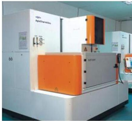
慢走丝车间 Slow-feed wire cutting workshop
