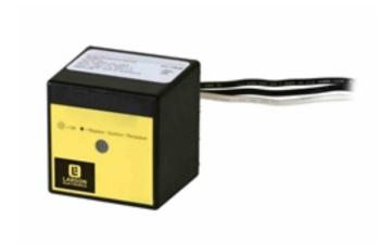
The Larson Electronics MT-SRG-T1SP-3PH-40KA-400Y.230-N4X Surge Protective Device actively protects electrical systems and sensitive equipment in rugged work sites. This Type 1 SPD is compatible with three-phase 400Y/230V AC Wyn-n, 50/60Hz and is rated at 40kA maximum surge current per phase. Equipped with green diagnostic LEDs, the NEMA 4X rated device is constructed of steel.
