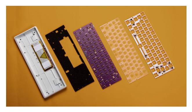
(Bottom Case > Sound Dampening Foam > PCB Board > Shallow Gasket Pad > Top Plate)
