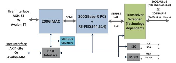
The 200Gbps Ethernet IP solution offers a fully integrated IEEE802.3bs compliant solution for use in core networks, Ethernet switching and network interface card (NIC) applications. The Ethernet cores implement an efficient architecture to achieve best in class resource utilization and performance numbers for targeting the complete 200Gbps Ethernet solution to ASICs as well as FPGAs.
