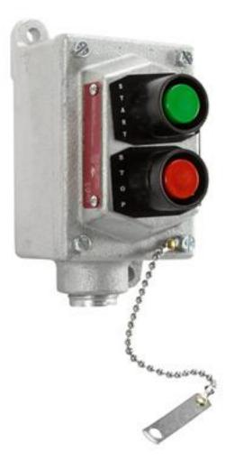
The Larson Electronics EPS-2XPB-SG-3P Explosion Proof Push Button Stop/Start Switch is Class I Divisions 1 & 2 and Class II Divisions 1 & 2 rated for Hazardous locations and UL 698 listed. This explosion proof switch provides manual starting and stopping of small AC and DC motors. The EPS-2XPB-SG-3P is for three phase current up to 250V.
