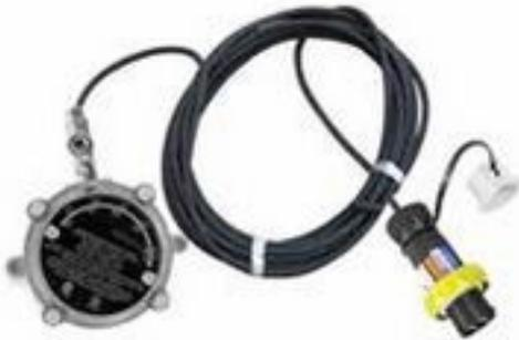
The Larson Electronics EXP-TSTAT-250V-86F-20M-CE16 explosion proof thermostat is designed for temperature control in industrial facilities where flammable gases, vapors or dust are or may be present. This device is adjustable using a set point knob system, which is powered by an SPDT snap action switch. Equipped with a 20-meter 16/3 SOOW cord and an explosion proof cord cap, the unit features a temperature limit range of -49°F to 176°F (-45°C to 80°C) and is rated at 250V AC (maximum).
