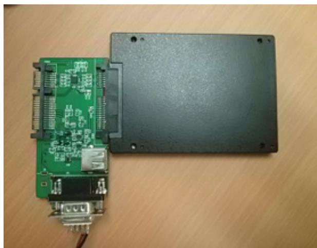
The test fixture has a DC-DC controller and a bus isolation circuit, and is controlled via a serial port connected to a PC. Special test code written by Cactus Technologies randomly shuts off power and isolates the interface bus from the DUT. This ensures that the DUT is not powered via interface bus signals.
