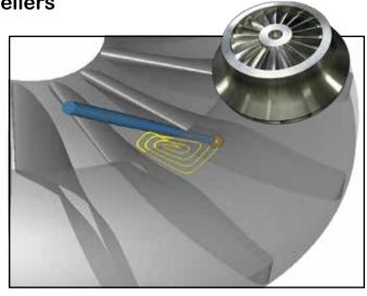
MAX-SI includes strategies for pocket roughing, plunge milling, box passes for finish/semi finish, and flow-direction finish milling.
