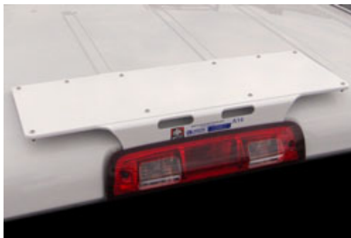
MMP-DC-RAM-2009-LED Steel Plate is Magnetic
