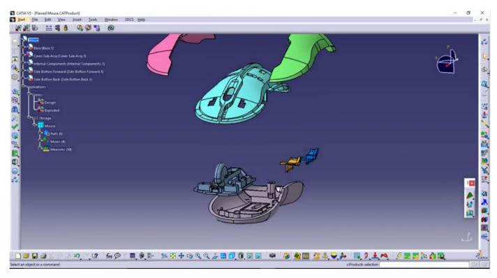
Digital GD&T improves the functions of integrated tools. Since the computer-based model includes all the needed data for development, it no longer relies on multiple human inputs, which naturally increase error. The products can therefore be created directly by manufacturers or even via 3D printer, since the 3D design is the only artifact in the process.
