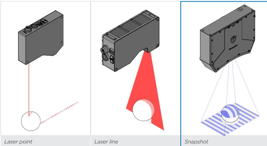
When choosing what type of sensor to buy, you can follow this simple rule of thumb: **laser profile sensors** are used to **scan moving targets**, while **snapshot sensors** are used to scan targets that are **momentarily stationary**.
