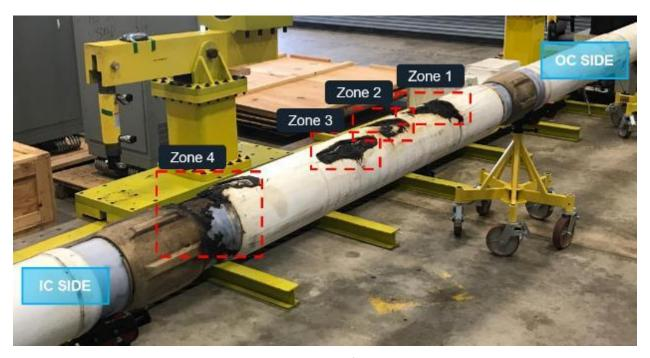
Figure 42: Isolator Damage from 2019 Restart
