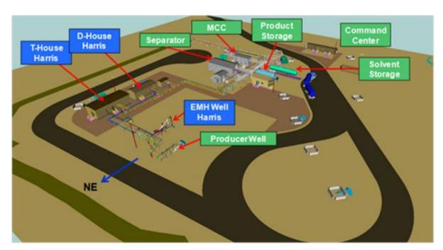
Figure 33: ESEIEH® Small Scale Pilot Facilities
