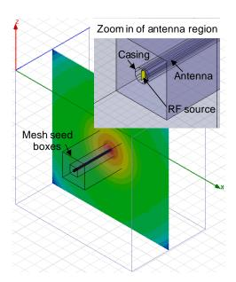
Figure 12: EM model of the antenna and oil sands
