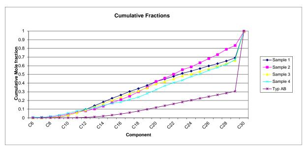
Figure 27: Sample compositions from the Mine Face Test produced fluid compared to **Athabasca Bitumen (Typical)**
