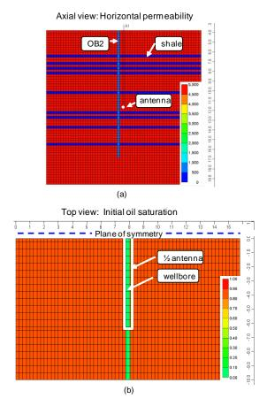
Figure 11: Reservoir model domain (a) axial view of horizontal permeability, (b) top view of initial oil saturation at the antenna elevation (distance units = m)
