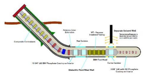
Figure 35: Revised Design - ESEIEH® Phase II Antenna/Injector (EZI-1)
