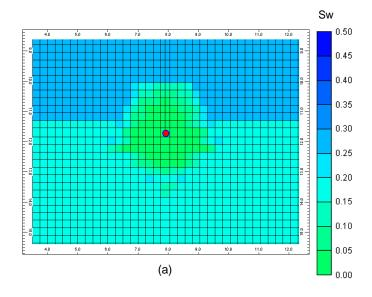
Figure 21: Predicted water saturation at day 33 from axial view at the antenna center (red dot marks the antenna position, distance units = m)
