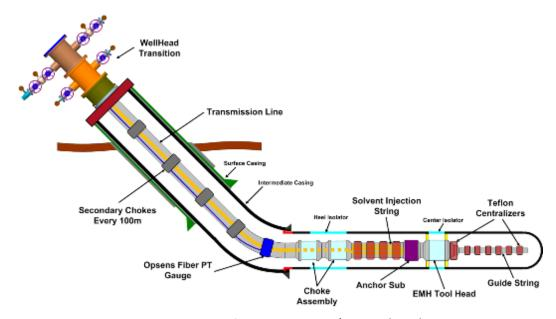
Figure 29: ESEIEH® Phase II Antenna/Injector (EZI-1)
