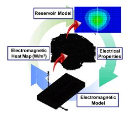
Figure 4: Graphical representation of the coupling between the EM and reservoir solvers
