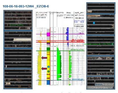
Figure 32: EZOB-6 Core and Well Pair Placements
