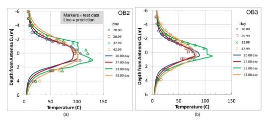
Figure 20: Comparison of the adjusted CEMRS model with test data from day 20 to day 43 (a) OB2, (b) OB3
