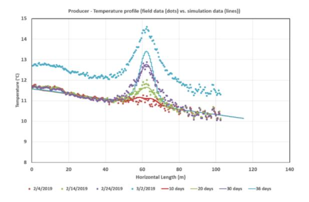
Figure 41: Producer Temperature Profile from 2019 Restart
