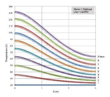
Figure 5: Comparison of CEMRS temperature profiles over a 10 day period compared to the MATHCAD® solution
