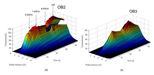
Figure 15: Surface plots of the temperature field evolution at the vertical a) OB2 and b) OB3
