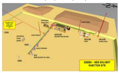
Figure 36: Revised Design - ESEIEH® Phase II Solvent Injection Site (EZI-2)
