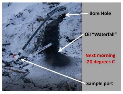
Figure 25: Sample from the borehole entrance transferred to another container. Sample temperature at the pour time was 4.5°C (40°F)
