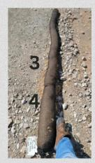
1, 2, 3, 4 depict the natural netting degradation of BioWorm<sup>™</sup> as a result of exposure to environmental factors, encompassing direct sunlight and repeated rainfall events.
